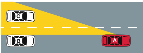
Using the left outside mirror, the driver of vehicle A can see vehicle C.
